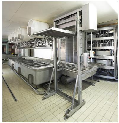
${\bf Atelier\ de\ fabrication:\ installations\ de\ soutirage\ et\ de\ pressage.}$
