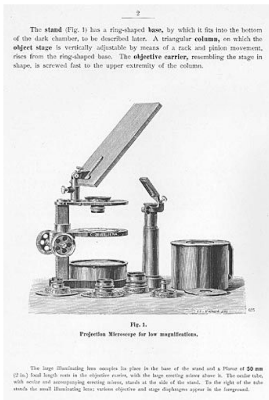
Projection Microscope for low magnifications, 1ère moitié 20e siècle.
