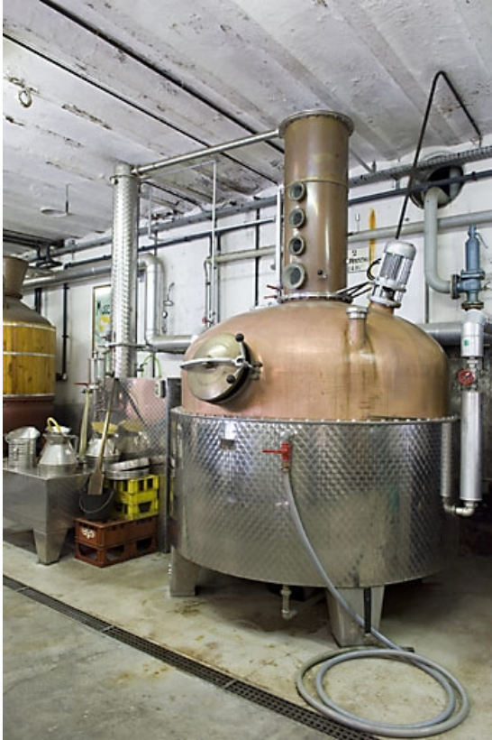
Atelier de distillation. Alambic Arnold Holstein.
