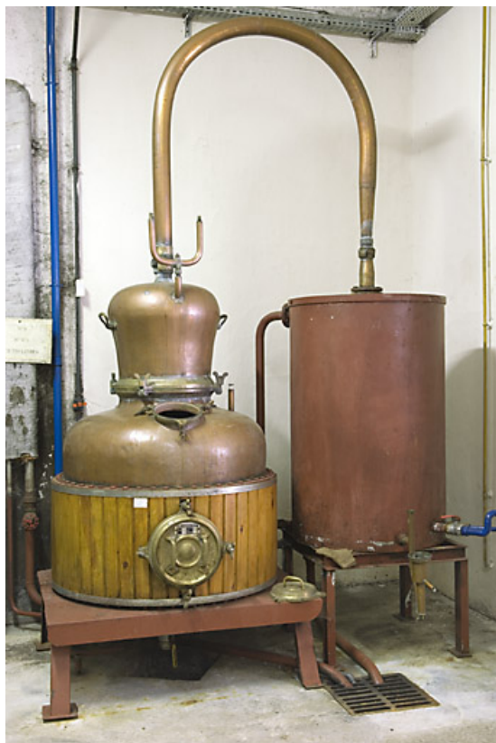
Atelier de distillation. Alambic Rump.
