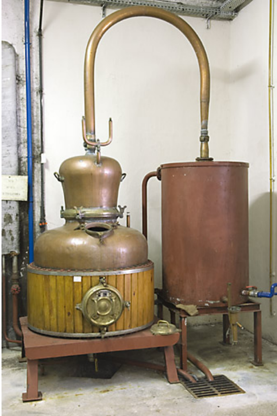
Atelier de distillation. Alambic Rump.
